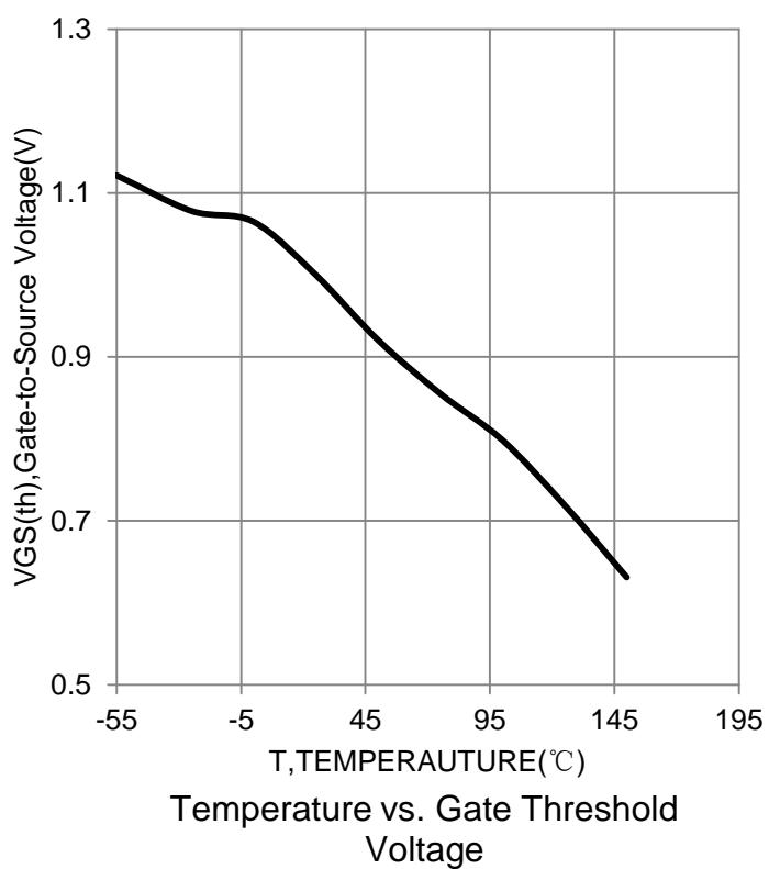
Temperature vs. Gate Threshold Voltage
